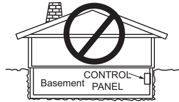
INCORRECT Locating Control Panel below earth level impairs range
